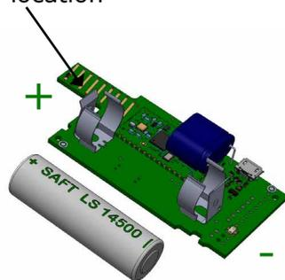
Disposition of the battery on the card
