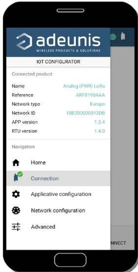
The IoT Configurator is a adeunis® application developed to facilitate the device configuration using a user-friendly interface. The IoT Configurator can be used on a smartphone or a tablet using Android or on a computer using Windows.
