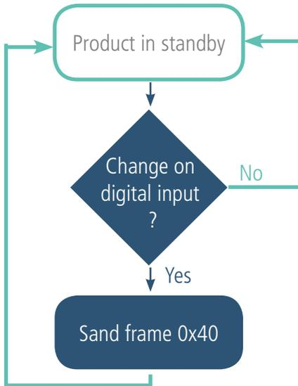
The product allows the transmission of a frame after a change of state on one of its inputs according to the following diagram:
