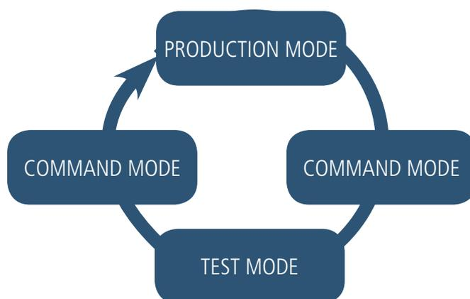
The return to the production mode is done by the ATO command or by disconnecting the USB cable
