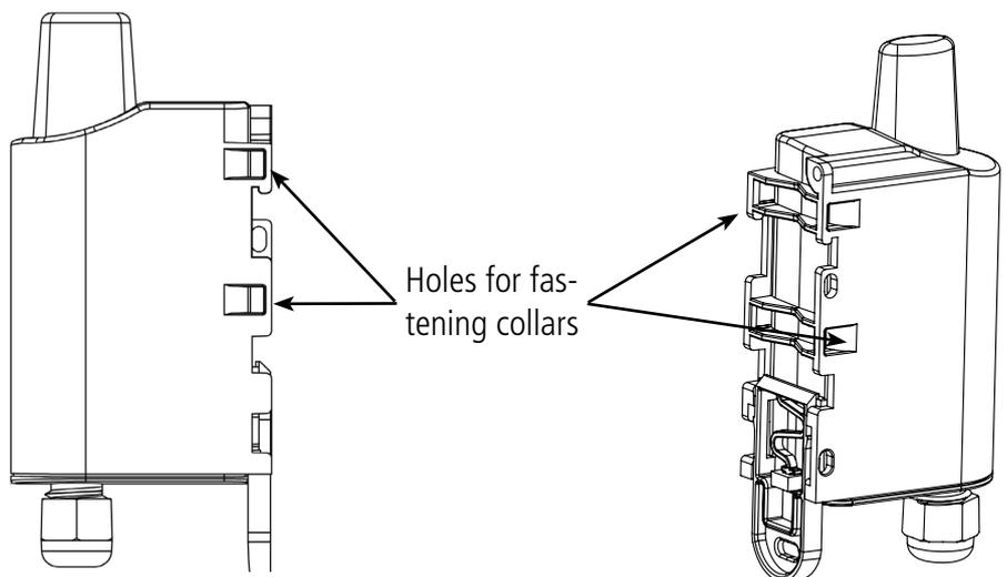
To optimize fastening onto a tube or mast, we recommend you remove the Rail-DIN locking/unlocking lever.
