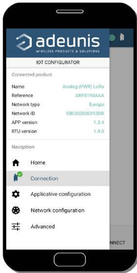
IoT Configurator is an adeunis® application developed to facilitate the configuration of devices through a user-friendly interface. The IoT Configurator can be used directly on a mobile or tablet in Android or via a Windows PC.
