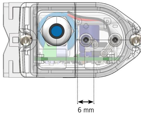
In order to ensure proper connection of the product, take care to connect the tube positioned where the pressure is highest on the P+ support (indicated on the base plate) and to connect the tube going into the section with the lowest pressure on the P- support.
