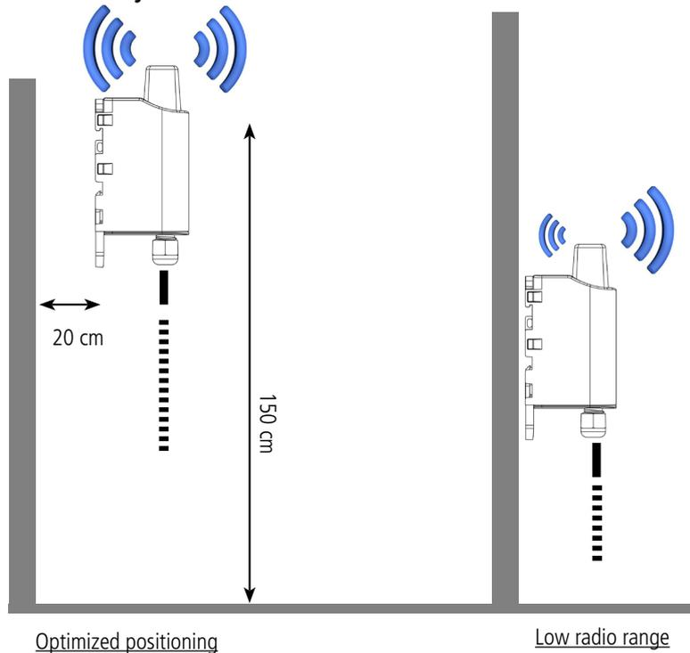
Since Air Handling Unit (AHU) are usually in enclosed areas or on roofs (Rooftop package unit), certain installation rules must be followed to ensure proper operation of the product:
